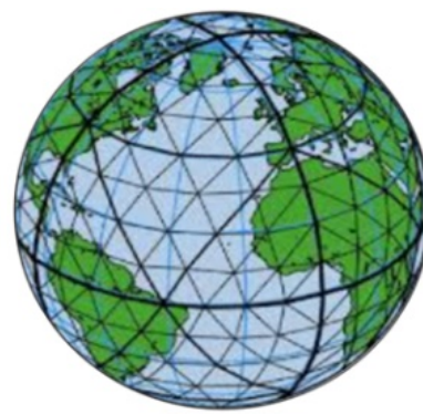
c) Triangular cells on QTM of an octahedron, levels 0–3 with refinement ratio of 4. (courtesy of Geoffrey Dutton)
